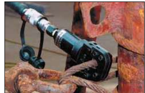
Steel rope is easily cut with the smooth guillotine action of an Enerpac cutterhead. ▶
